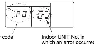
**2** Every pushing of
