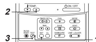
**1 When **SET** and **TEST** buttons are pushed simultaneously for 4 seconds or more, the following display appears.**
