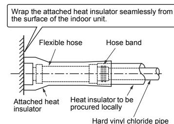
\* Direct the slits and seams of the heat insulator upward to avoid water leakage.
