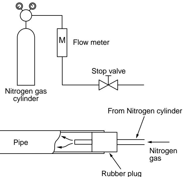
Fig. 7-5-1 Prevention of oxidation during brazing
