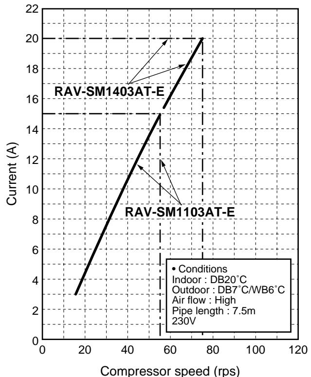
• Operation characteristic curve <Super Digital Inverter>
