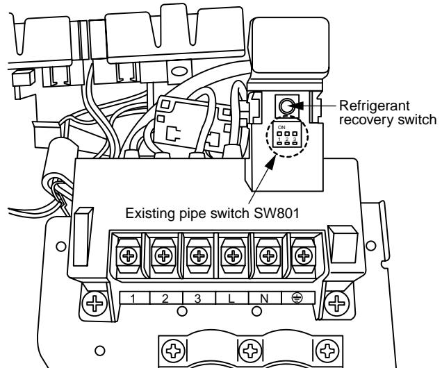
Only when the existing gas pipe Ø19 mm is used on RAV-SM803AT-E model, change the setting of SW801 No. 3.
