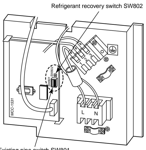
Only when the existing gas pipe Ø19 mm is used on RAV-SM1103AT-E model, change the setting of SW801 No. 5.
