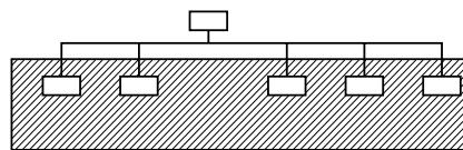
(2) When there is an effective opening with the adjacent room for ventilation of leaking refrigerant gas (opening without a door, or an opening 0.15% or larger than the respective floor spaces at the top or bottom of the door).
