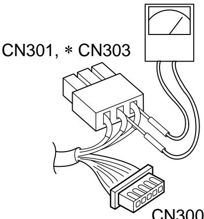
CN300 : Motor coil winding
