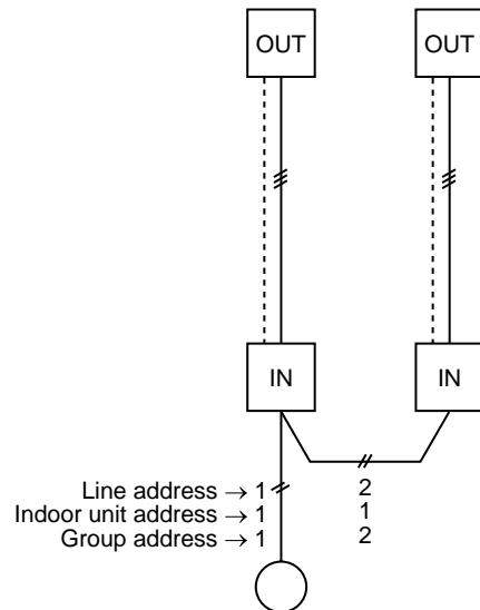
For the above example, perform setting by connecting singly the wired remote controller without remote controller inter-unit cable.
