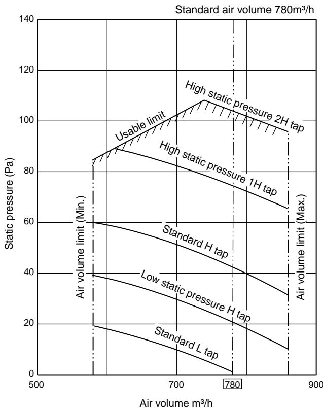
Fig. 3 RAV-SM802BT-E (Round duct)
