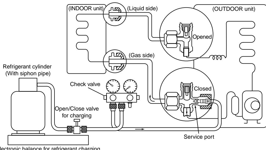
Fig. 7-4-1 Configuration of refrigerant charging
