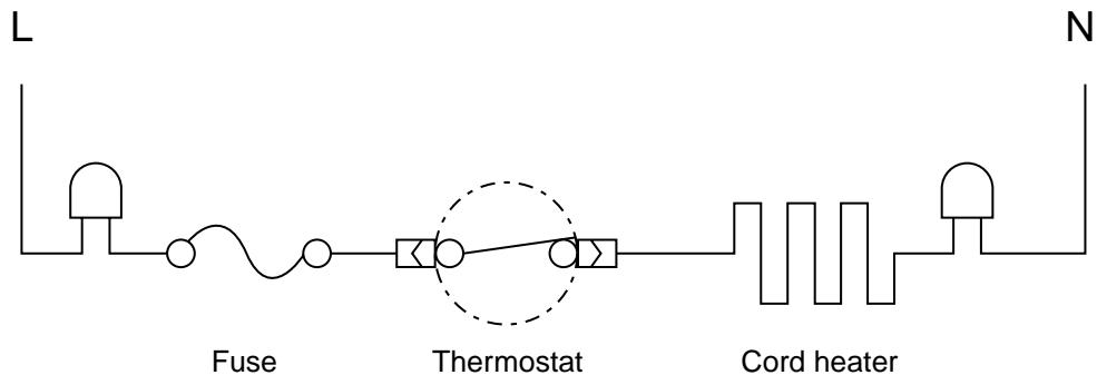
\* Be sure to connect the fuse and the thermostat to LIVE side of the cord heater.
