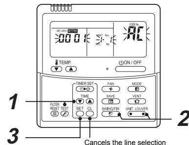
If no number appears on UNIT No., no outdoor unit exists on the line. Push
