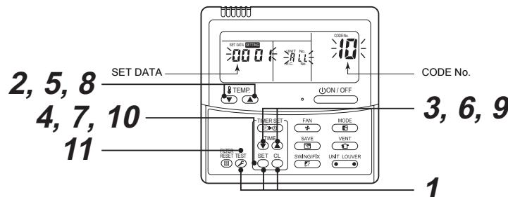
Pair the indoor unit to set and the remote controller one-to-one.
