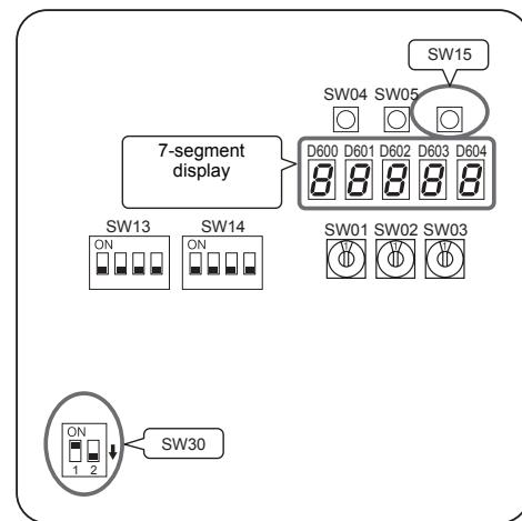
**Switch setting (setting example when controlling 2 or more refrigerant lines centrally)**
