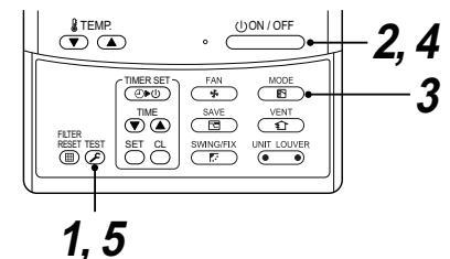
**1** Push and hold the **TEST** button for more than 4 seconds. TEST appears on the LCD display and the unit enters the trial mode. (TEST is indicated on the LCD display during the test run.)
