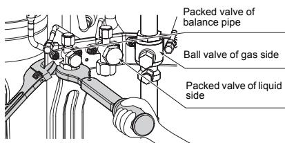
**Pipe connection method of valve at the gas side (Example)**
