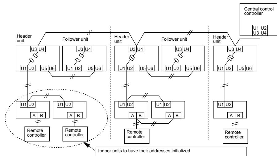
**2** Turn on the indoor and outdoor units of the refrigerant line for which you want to initialize the addresses. About one minute after turning on the power, confirm that the 7-segment display on the header outdoor unit indicates "U.1. - - -" and operate the interface P.C. board on the header outdoor unit of the refrigerant line as follows.
