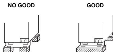
4. Mount the vibration-proof rubber (including vibration-proof blocks) so that it fits under the whole clamping leg.
