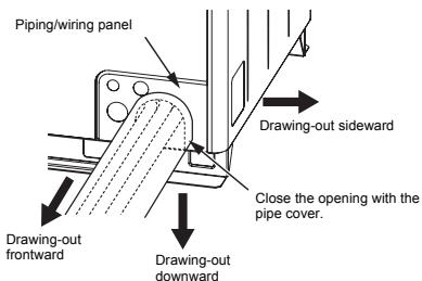
**When not using the piping cover**
