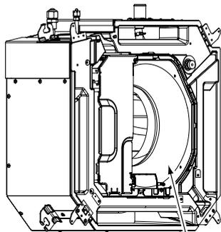
Be sure to remove the cushion for transportation between the fan and the bell mouth.
