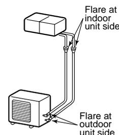
Align the centers of the connecting pipes and tighten the flare nut as far as possible with your fingers. Then tighten the nut with a spanner and torque wrench as shown in the figure.
