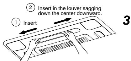
Be careful to insert the louver in the correct direction.
